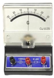
• The arrow on a galvanometer deflects depending on the amount of current passing through.
